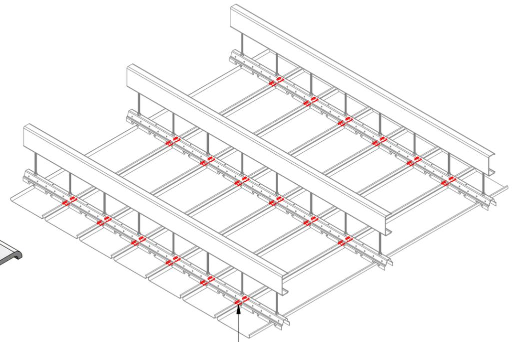
Seismic Clip at every point of contact between Panel and Carrier.
