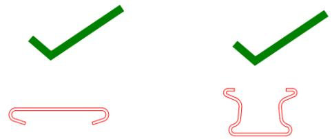
**Note:** Seismic Clip can be used with both Recessed Filler Strip and Flush Filler Strip
